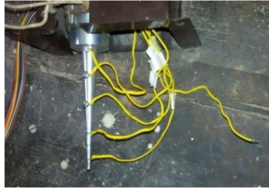
Figure 6: Conical Spine Connect to Heater of Apparatus
