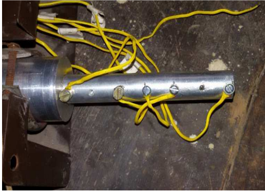
Figure 5: Cylindrical Spine Connect to Heater of Apparatus
